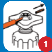
Remove handwheel pin.
