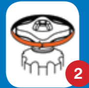
Turn handwheel anti-clockwise one turn.
