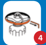
Close valve tightly and remove steel wire.
