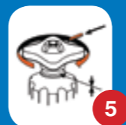
Turn handwheel clockwise until sleeve seats on bonnet rim and re-insert handwheel pin.
